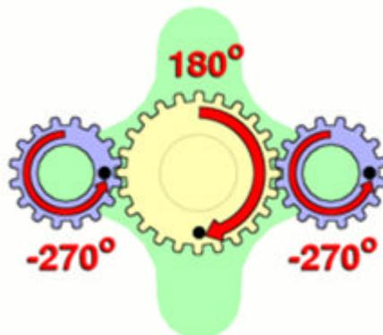
*The carrier (green) is held stationary while the sun gear (yellow) is used as input. The planet gears (blue) turn in a ratio determined by the number of teeth in each gear. Here, the ratio is  $-24/16$ , or  $-3/2$ ; each planet gear turns at  $3/2$  the rate of the sun gear, in the opposite direction.*
