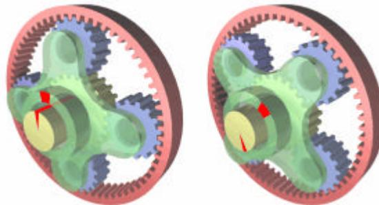
*Epicyclical gearing is used here to increase output speed. The planet gear carrier (green) is driven by an input torque. The sun gear (yellow) provides the output torque, while the ring gear (red) is fixed. Note the red marks both before and after the input drive is rotated  $45^\circ$  clockwise.*
